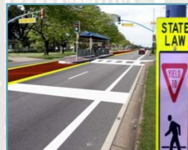
Mid-block pedestrian crossing with overhead signals at a transit station
