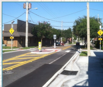
Rectangular rapid flashing beacons at midblock crossing (Orlando, FL)
